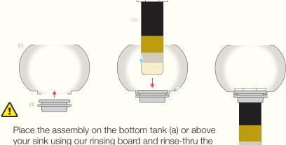
equivalent of 2 tanks (b) or 8 liters of water. Do not forget to rinse the bottom tank if you opt for the first
