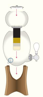
You can now start the filtration process of your OVOPUR unit by filling the upper tank using a pitcher. The magnetic disc (g ') of the magnetic gauge (g) indicates the water level inside of the tank. The virtual horizontal line drawn by the end top of the handle of the tap indicates the point from which you can reload the filtration tank at full capacity (4L) without fear of overflowing.
