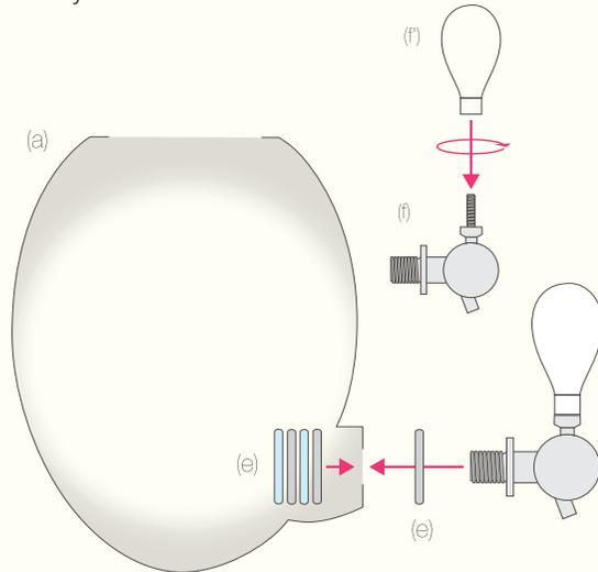
Screw in the inner nut (h) until it presses the stainless steel and silicone gaskets together against the ceramic wall, hold with your hand and perform the last turn clockwise with the tap using your other hand until it firmly holds in place.
