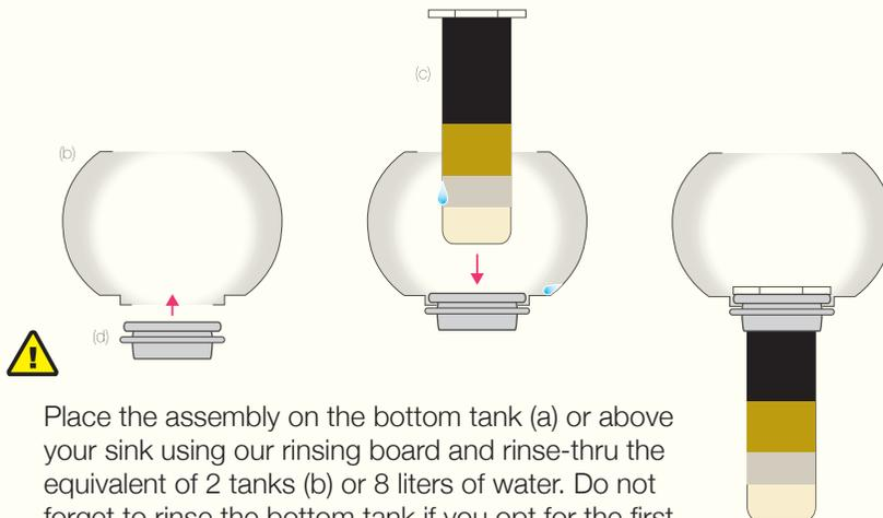
Place the assembly on the bottom tank (a) or above your sink using our rinsing board and rinse-thru the equivalent of 2 tanks (b) or 8 liters of water. Do not forget to rinse the bottom tank if you opt for the first option.
